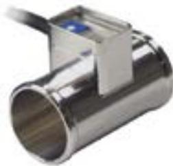
An adjustable thermostatic fan control specially made to control all 12 volt fans. Made from billet aluminium, it fits into your radiator hose and is secured with two hose clips ensuring a perfect seal. Latest surface mount sensor with no mechanical parts to wear or fail. Simply adjusted with a screwdriver to bring in the radiator fan between 70 and 120°C. Supplied with 2 hose clamps, 30 amp relay, cap, 3 cable ties, 1 x self tapping screw and fitting instructions
