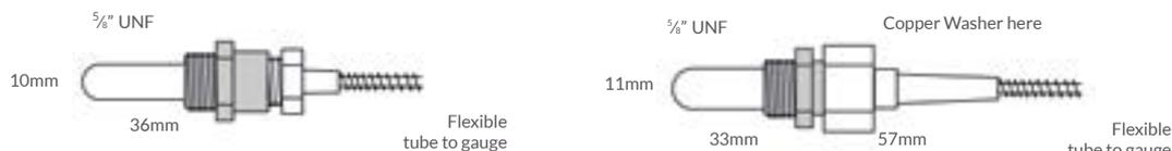
Electrically operated temperature gauges require a sender which screws into the head or block:
