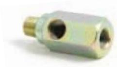
Enables you to fit a mechanical or electrical gauge and retain your original oil pressure switch. These adaptors fit in place of your original oil pressure switch which is then screwed into the end of the adaptor. The side take-off 'B' is tapped 1/8" NPTF (27 t.p.i.) into which you can fit Oil Pressure Adaptor **070.031** for mechanical gauges or Oil Pressure Sender **070.185** for electrical gauges
