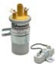
12 volt high energy coil for use with Lumenition Electronic Ignition Systems to get the best performance from those systems. Must be used with the ballast resistor supplied unless already fitted on the car. 12 volt with push in lead. Overall height 150mm, body height 100mm, diameter 50mm, primary coil resistance 1.4 ohms and secondary coil resistance 7.0 k/ohms. The mounting bracket for the coil is included
