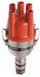
123 Ignition Distributors replace most LUCAS distributors for engines in British cars. 6 or 12 volt, positive or negative earth unless specified. They offer 16 different advance-curves that can be selected via a little switch which enables you to fine tune your engine. They also offers automatic dwell, spark balancing, automatic power cut off one second after engine stops. There are dedicated 123 Ignition Distributors for specific makes and models.
