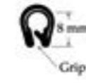
PVC EDGE TRIM - 8mm Grip range 1mm to 2mm. Goes 8mm over flange. Black 060.212
