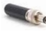
LOCKING PLUG Max load 5 amps at 12V. Ferrule screws on to socket 080.650 to stop it falling out. Black only 080.653
