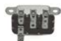
LUCAS 33135 NORMALLY OPEN HORN RELAY SB40 LUCAS 33135/SB40 type relay. A Relay is an electrical switch which uses low wattage current to open another switch. It is this second switch that carries and switches the high wattage current. This is a general purpose Relay in a metal case with two fixing holes and features screw connections for your wires. It is normally open and operates on 12 volts and up to 20 amps for horn, lights etc. This type of relay was fitted to XK Jaguars and early DB Series Aston Martin and many other applications 33135/SB40
