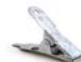
LUCAR FITTING 76mm long with a 32mm jaw opening and a 6.4mm lucar connection for the lead. Maximum recommended load is 25 amps. Plated steel 080.016
