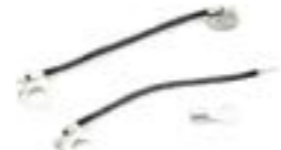
LOW TENSION LEAD SET For LUCAS DVX4A and DVX6A distributors. One terminal is supplied loose because it is necessary for you to pass the wire through a small hole into the distributor and then fit the terminal 030.085
