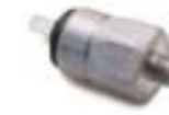
ADJUSTABLE 0-16 P.S.I. Switches on when oil pressure drops below the set figure which can be adjusted between 0 and 1.1 bar (16 p.s.i.). Diameter 26mm with 1/8 in NPTF thread 020.127
