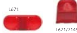
RED LENS L671 As fitted to Volvo P1800 for L671 Rear lamp L671 The red lens only for the L671 rear lamp fitted to the Volvo P1800 L671/7145
