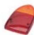
REAR LENS L801 Red and Amber Stop, Tail & indicator lens only. Fitted to Jaguar XJ6 S1, XJ12 S1, and Daimler Sovereign L80154580348 LH Clear Lens L80154580349 RH Clear Lens
