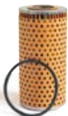
71mm PAPER OIL FILTER Paper filter element, 71mm dia, height 153mm. Jaguar 2.4-4.2 6cyl., Lancia Fulvia 1200/2C, 1300S, 1600H 016.403/2
