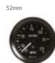
WATER TEMPERATURE Mechanical, 30 to 120°C. 3,048mm (120") capillary length 070.444
