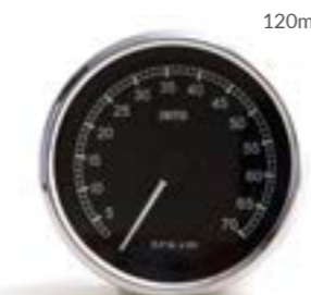
TACHOMETER Reads 0-7,000 rpm. 120mm diameter with full V chrome bezel, white figures on a black dial reading to 7000 rpm. Operates electronically from 12 volts and can be switched for 4, 6 or 8 cylinder engines. With 12 volt illumination. Requires hole size 120mm diameter. Depth over fixing studs 77mm 070.422
