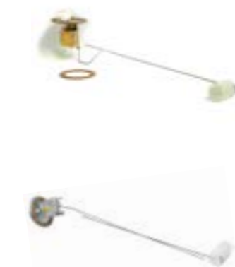
TOP MOUNTING SENDER Standard SMITHS fitting six holes 5.08 mm diameter on 60.33 mm pitch circle diameter. Gasket supplied. The arm length is adjustable for rectangular and cylindrical tanks of depths/diameters between 203 mm and 610 mm. After adjustment the arm is secured by soldering. Fitting and wiring instructions are provided. You will need to run a wire from the Sender to earth 070.011
